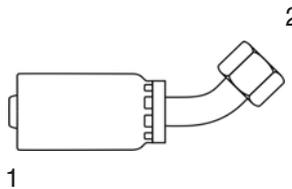
**Hose x FORFS SW 45 DEG Elbow Crimp Fitting**
