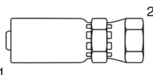
**Hose x FEM Air Brake SW Crimp Fitting**
