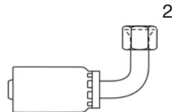
**Hose x FSAE SW 90 DEG Elbow Crimp Fitting**
