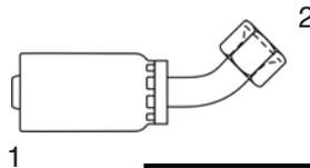
**Hose x FSAE SW 45 DEG Elbow Crimp Fitting**
